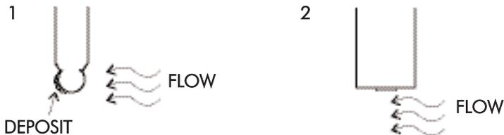
Exposed electrode surface will foul and require frequent cleaning.
