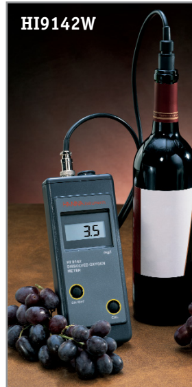
The HI 9142W and HI 9143W can be calibrated with no chemical solutions
