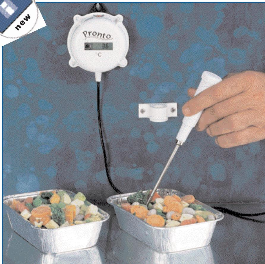
HI 146-00, HI 146-01 and the new waterproof HI 146-99 are high accuracy thermometers with a professional probe and a 2 meter (6.6') cable. They also incorporate the exclusive Cal-Check feature which allows you to double-check the accuracy of the meter any time.
