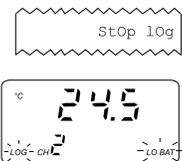
Note: When an external adapter or new batteries are connected, the printing must be manually enabled in order to return to logging with printing mode.
