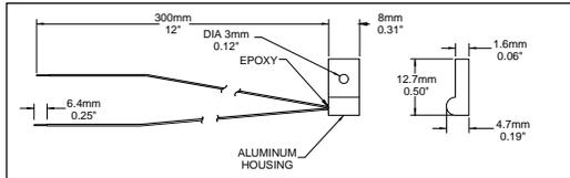
HI 76S2-6 NTC Thermistor sensor. PVC encapsulated tip for protection in aggressive environments.
