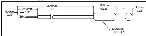
HI 76S2-7 NTC Thermistor sensor. Can be housed and used in any custom application.
