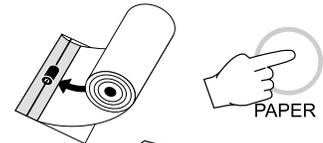
Allow about 5 cm (2") of paper to exit from the printer and replace the paper cover.
