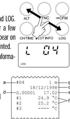
Note: If no keys are pressed, the meter enters standby mode to prolong the battery life and only the "LOG" indication will be visible on LCD. While timed printing during the sleep mode, the last printed reading will appear briefly on the LCD. To reactivate the LCD press ON/OFF.
