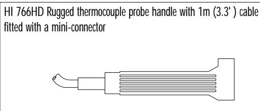
WITH INTEGRAL HANDLE, 1 m CABLE & MINI-CONNECTOR
