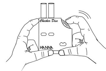
Note: A concentration of Chlorine above 50 ppm causes interference inhibiting the development of the color. In this case require the HI 3882/O Test Kit.
