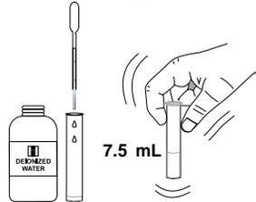
22- Remove the cap and add 1 packet of HI 93713-0 Reagent. Replace the cap and shake vigorously for 20 seconds. This is the reacted sample.
