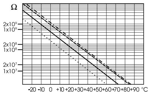
Since the resistance of the pH electrode is in the range of 50-200 Mohm depending on the composition of the glass, the current across the membrane is in the pico Ampere range. Large currents can disturb the calibration of the electrode for many hours.
