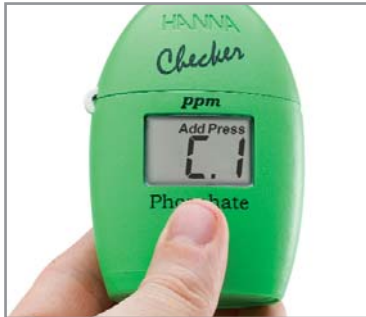
"Zero" the Checker®HC with your unreacted water sample
