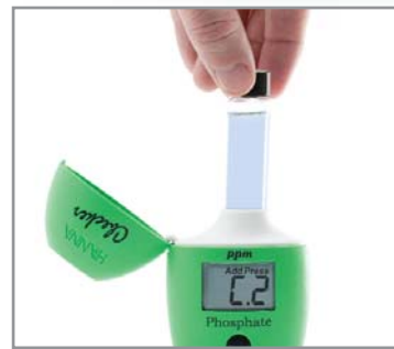
Place the vial into your Checker®HC
