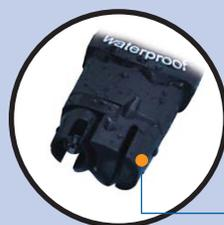
The graphite conductivity electrode provides greater accuracy because it does not get dirty from salt deposits in the solution.
